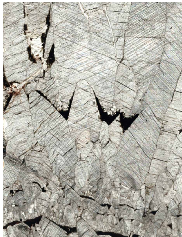
Figure 3: Thin-section image of carbonate cement growing near-instantaneously from clast (dark red, at base) into the open fracture. The image is about 2 cm wide.
